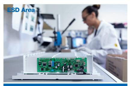
Free of electrostatic discharge area dedicated to the assembly and testing of electronic components.
